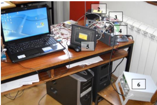
Fig. 4. Vibration measurement and simulation system
