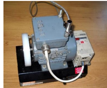
Fig. 5. Motor with an overhang disk
