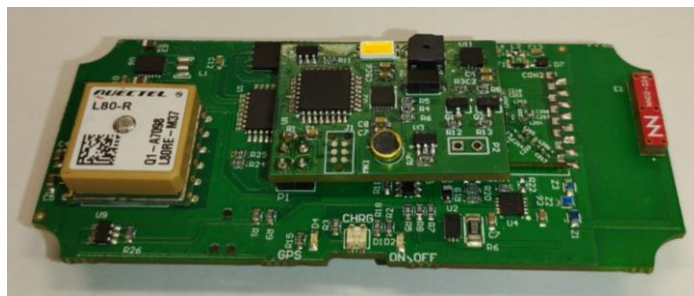
Fig.13. Dog collar system with the stimulation board extension
